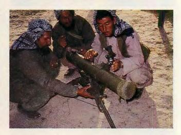
ABOVE: Chinese BM-12 single 107mm rocket launcher. Chinese are also manufacturing a single tube 122mm rocket launcher. Photo: Robert K. Brown
